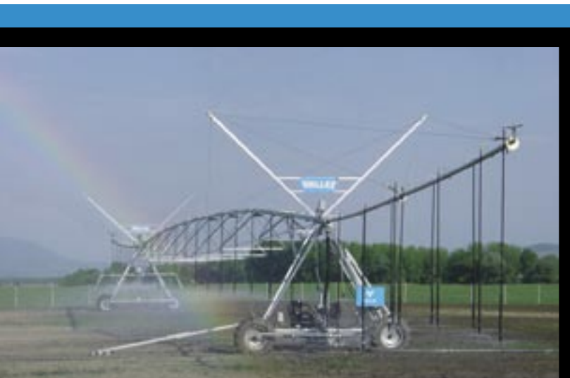
The Two Wheel Linear can cover adjacent fields by traveling down one side, then pivoting 180° and reversing direction to cover the other side of the field.
