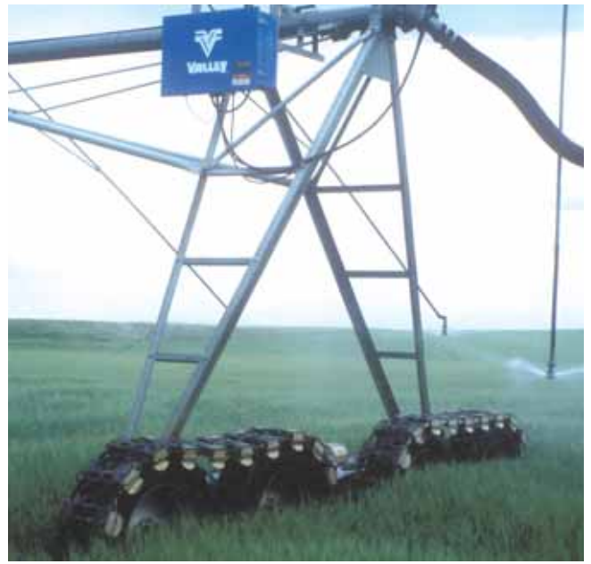
Valley® Spider™ Dual drive tracked option for increased floatation.
