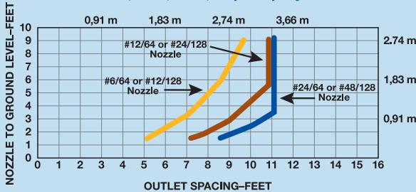
When nozzle is placed on drops
